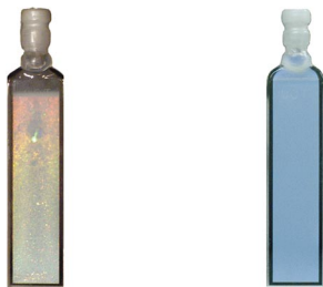
FIG. 1. (Color) Pictures of samples B (left) and F (right). The photograph was taken on the 161st day after the dispersion was introduced into the cuvette. Although sample B shows iridescence, the appearance of sample F indicates that no crystallization took place.
